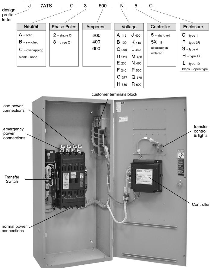
260 amp. size in typical enclosure with location of customer connections
